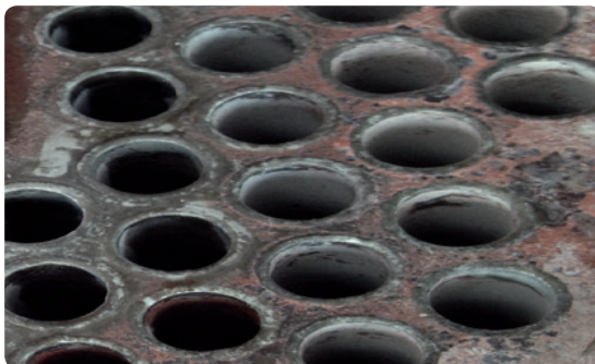
Conventional wastewater evaporators get dirty quickly. This results in reduced capacity and higher energy consumption.
