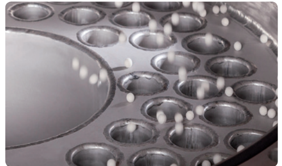
The self-cleaning Activepowerclean heat exchangers stay clean due to circulating grinding balls.
